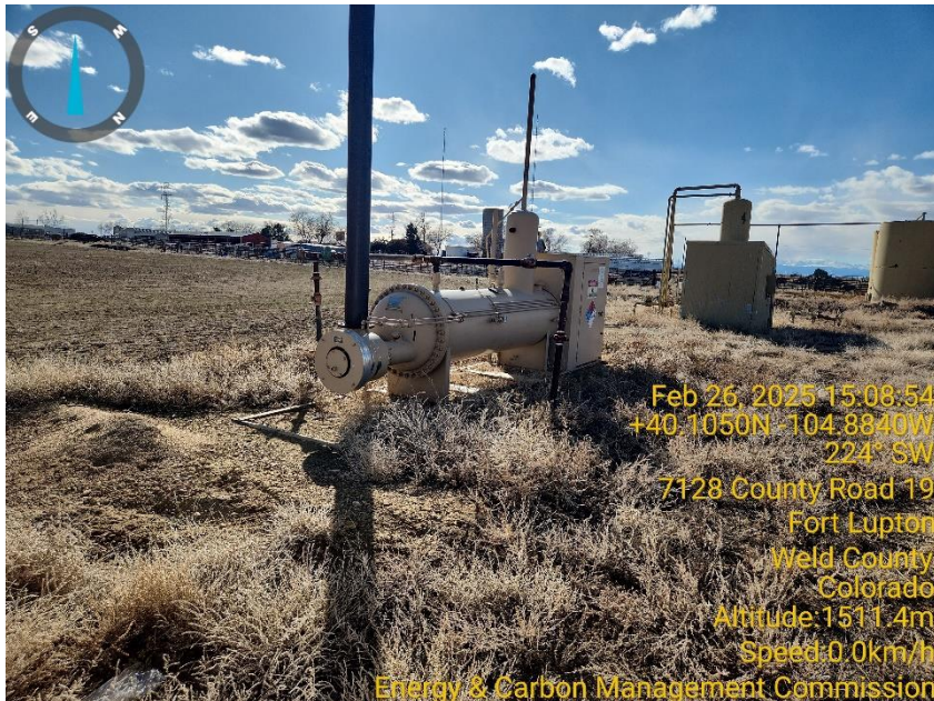
Photo 7 Horizontal heated Separator.
