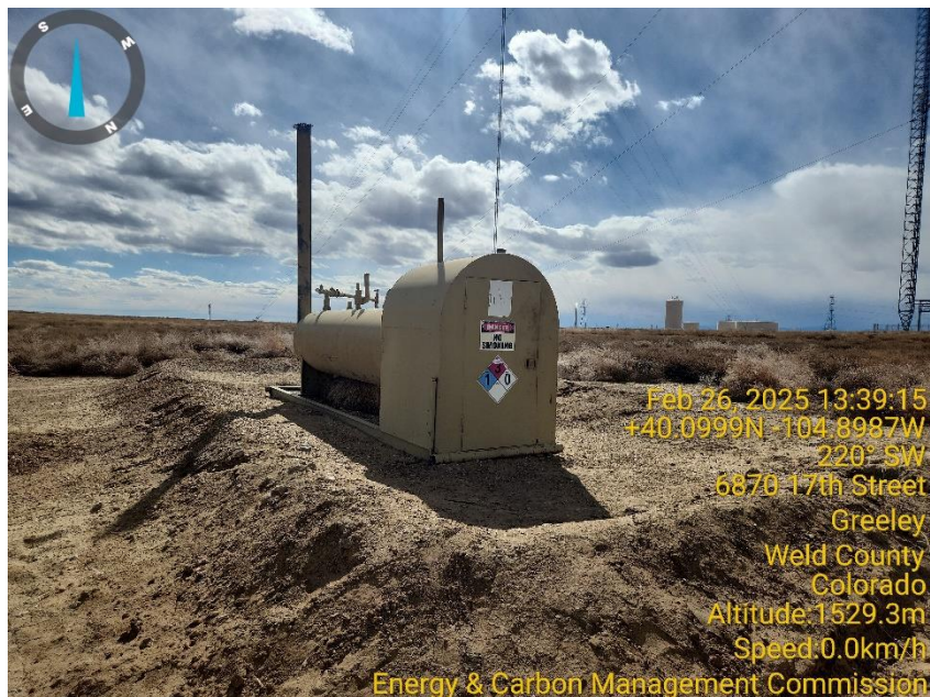
Photo 5 Horizontal Heated Separator.
