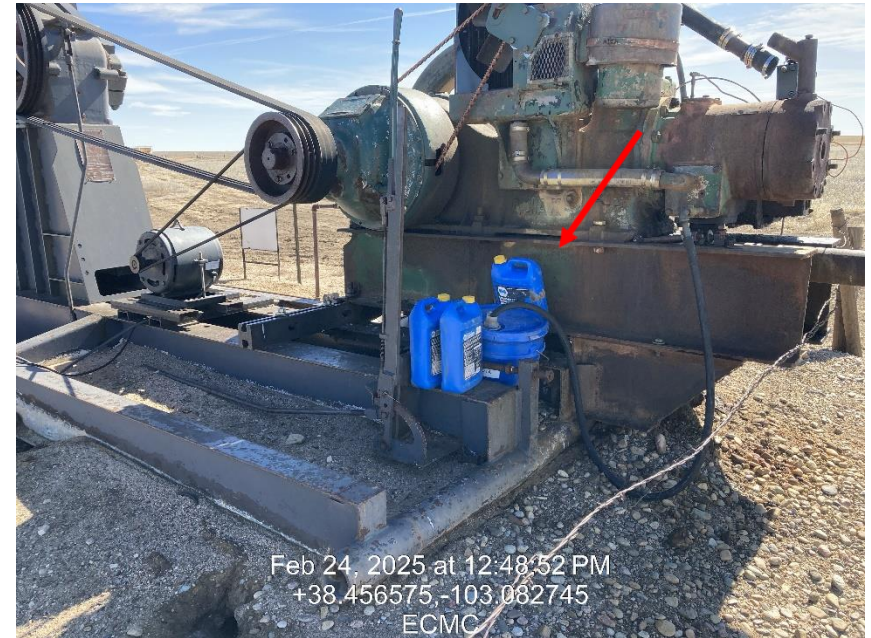
Photo 4 – Lube oil not in containment
