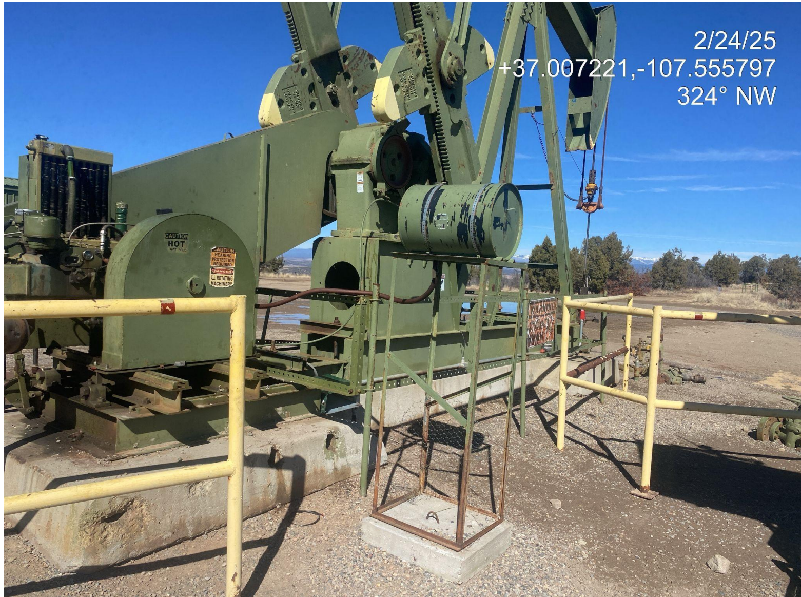
Photo 2. Oil/lube container at pump jack has no spill prevention/secondary containment.
