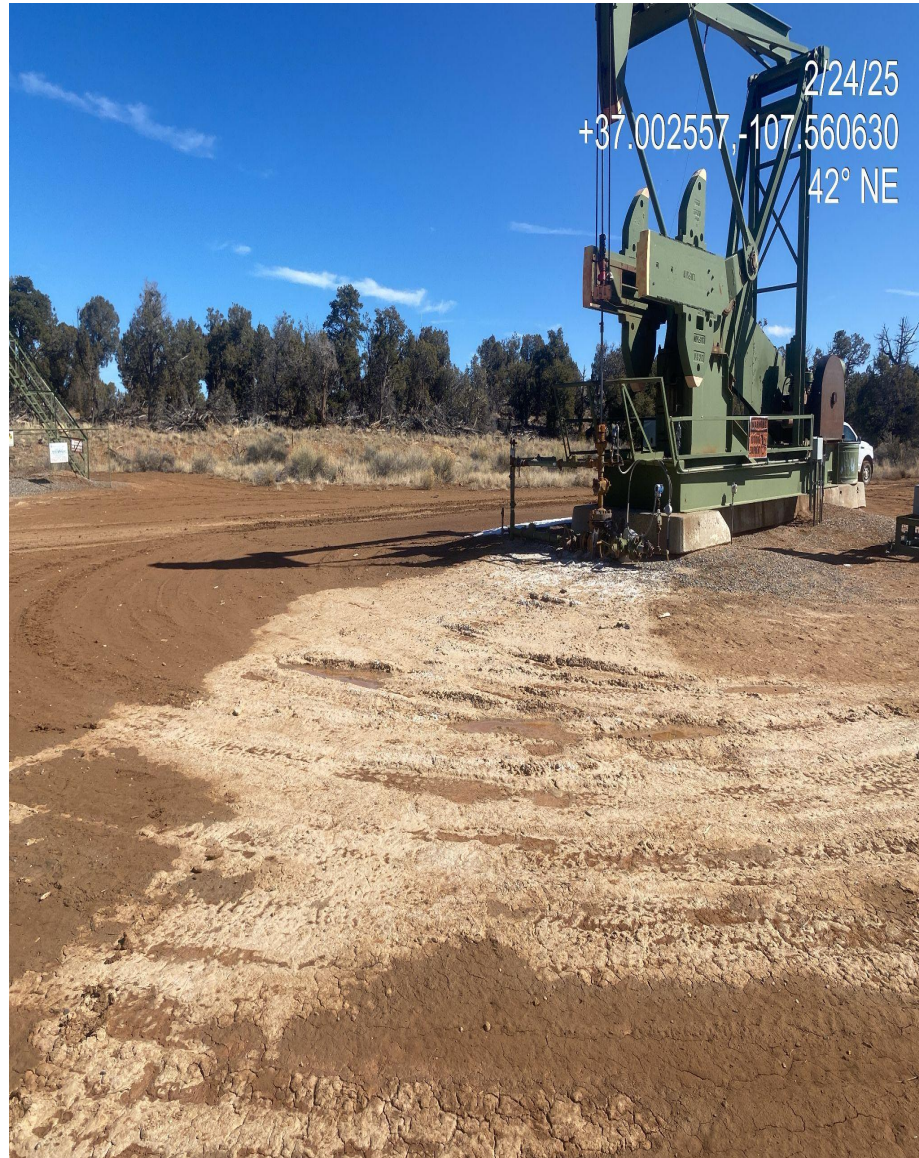
Photo 3. View of salt stain migrating from wellhead.
