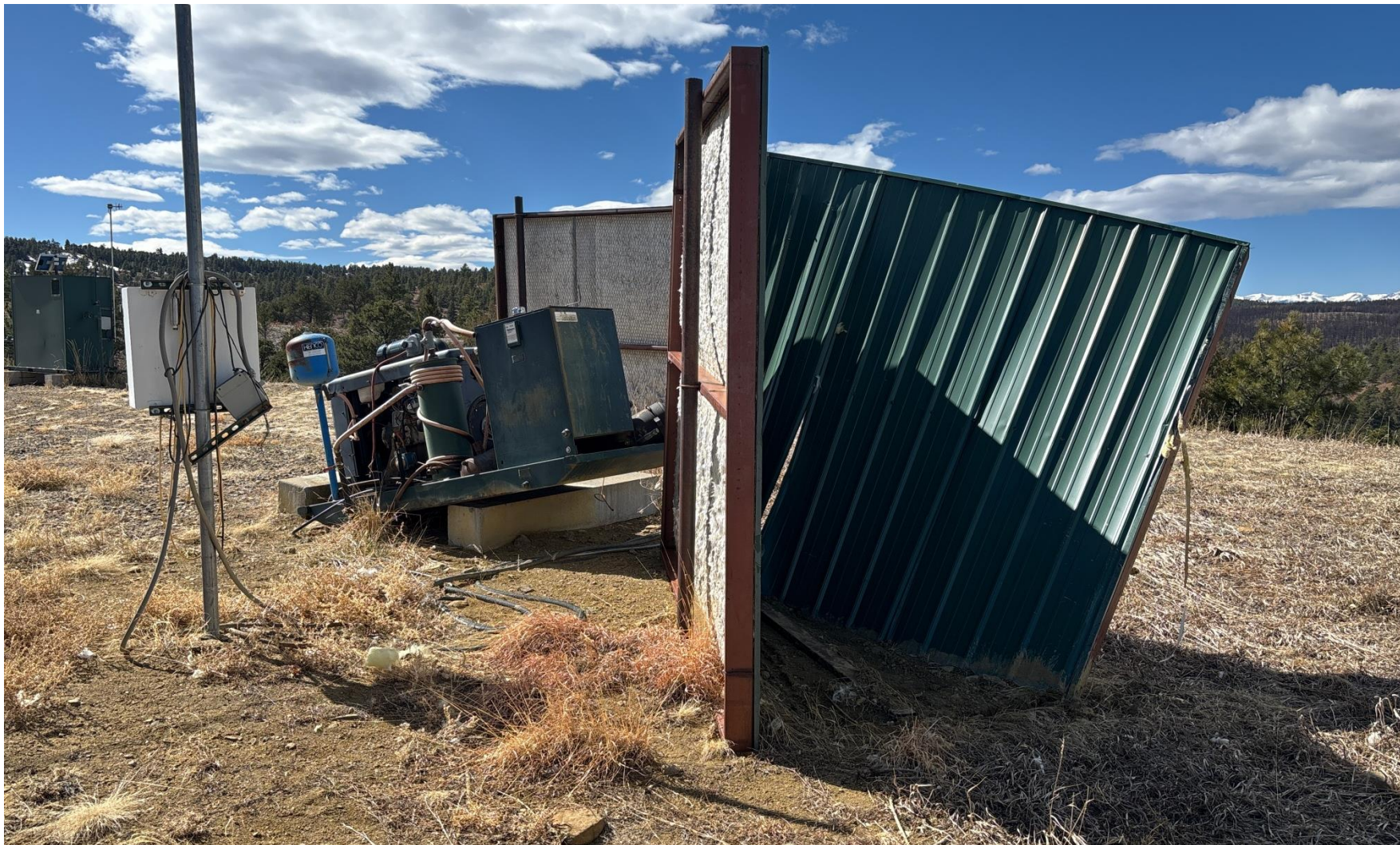
PHOTO 6: WELL HAS BEEN CONVERTED TO A SEISMIC MOTOR WELL SO ENGINE SKID AND SOUND WALLS ARE NO LONGER IN USE OR USEFUL TO THE OPERATION. REMOVE UNUSED EQUIPMENT PER RULE 606. CA DATE 3-4-2025.
