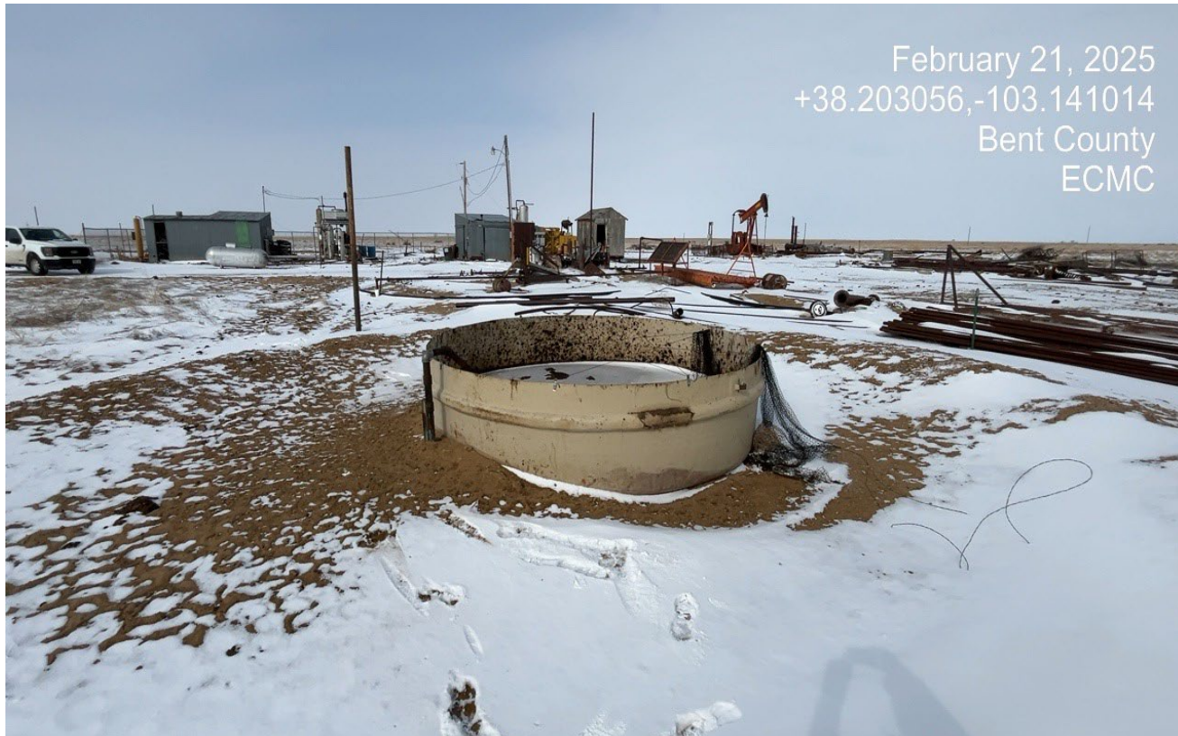
Photo 16. Facing northwest at the south side of the location. There is an open top fiberglass condensate tank with no wildlife or livestock protections. There are cattle tracks all around the tank indicating that cattle could be drinking out of this tank.
