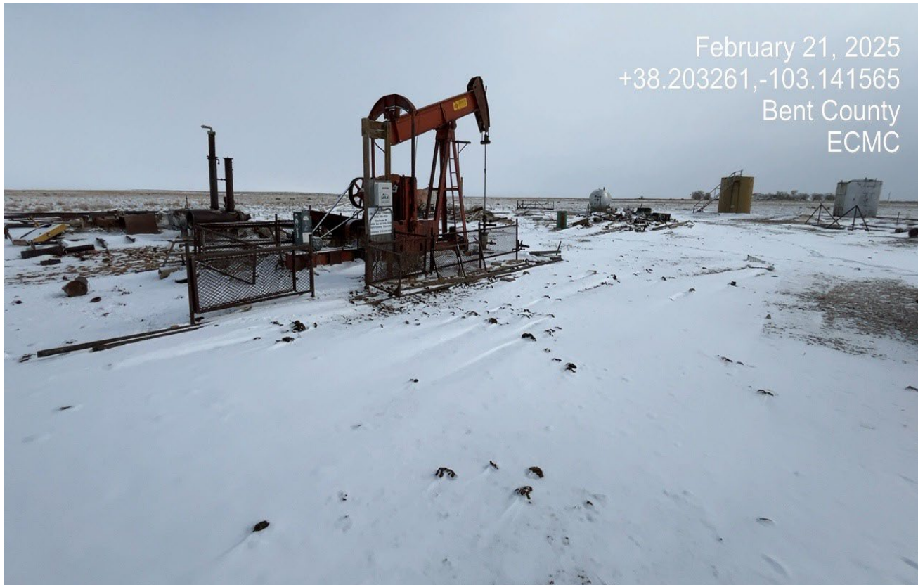
Photo 11. Facing northeast toward the well. The fence around the pumpjack is in disrepair and there is unused equipment stored near the well.
