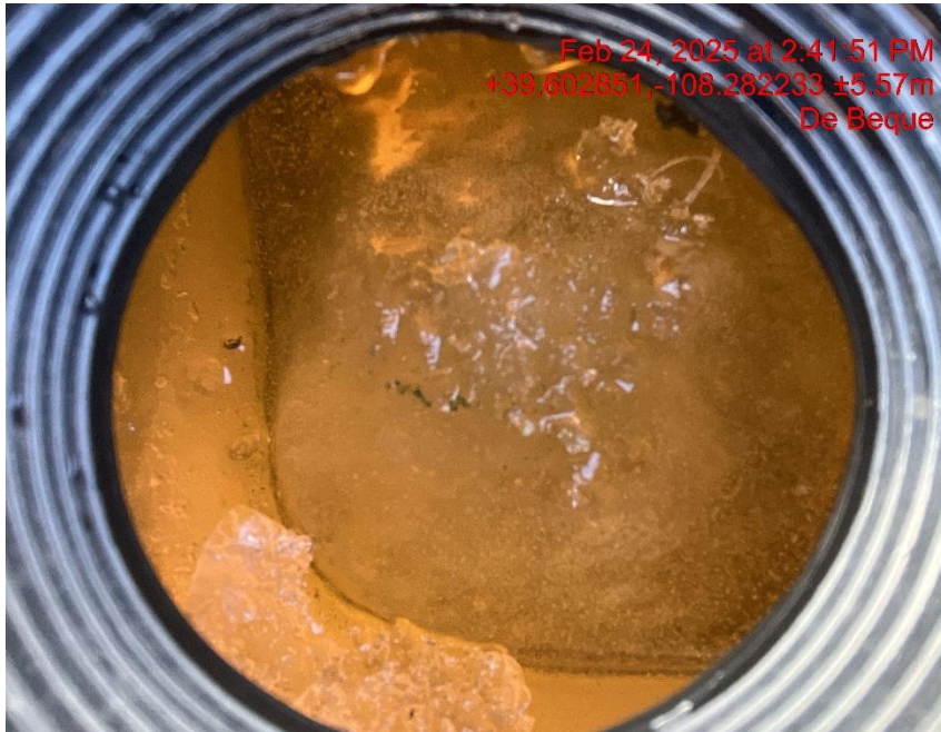
Photo # 5750 Failure to maintain chemical BMP's/chemical containments full of fluid & not sufficient to contain possible spill
