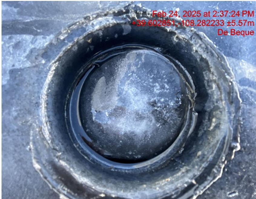
Photo # 5748 Failure to maintain chemical BMP's/chemical containments full of fluid & not sufficient to contain possible spill
