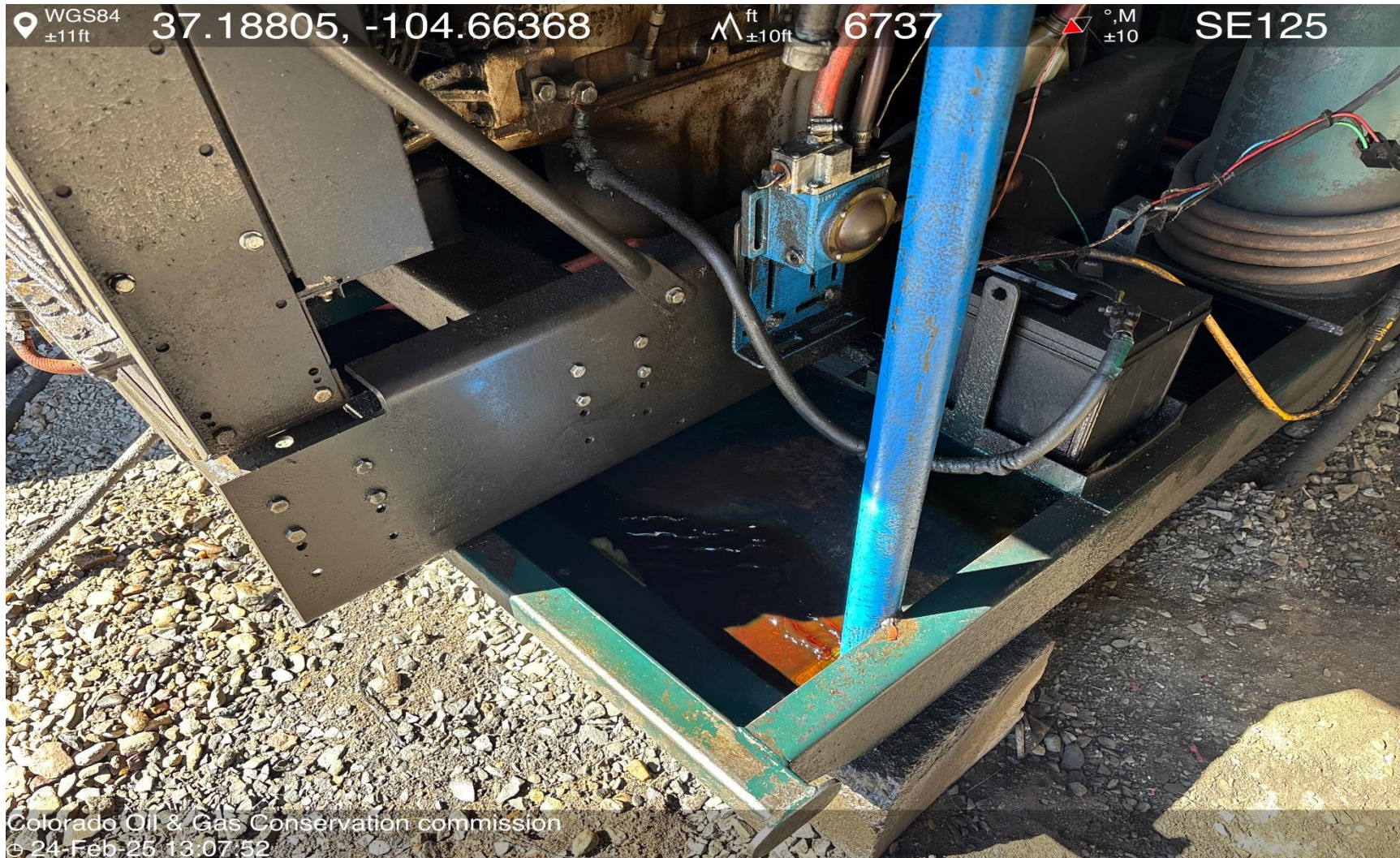
PHOTO 5: OILY WASTE IN ENGINE SKID. PHOTO 6: LEAKS ON COMPRESSOR MOTOR AND EQUIPMENT. Conduct maintenance on equipment, cleanup stained material and review self inspection processes. PER RULE 1002,(2).D. Comply with general provisions of the oil and gas act for wildlife protection AND SB-181. THIS IS THE SECOND NOTICE FOR THIS CA IMMEDIATE ACTION IS REQUIRED, EQUIPMENT MUST BE REPAIRED.
