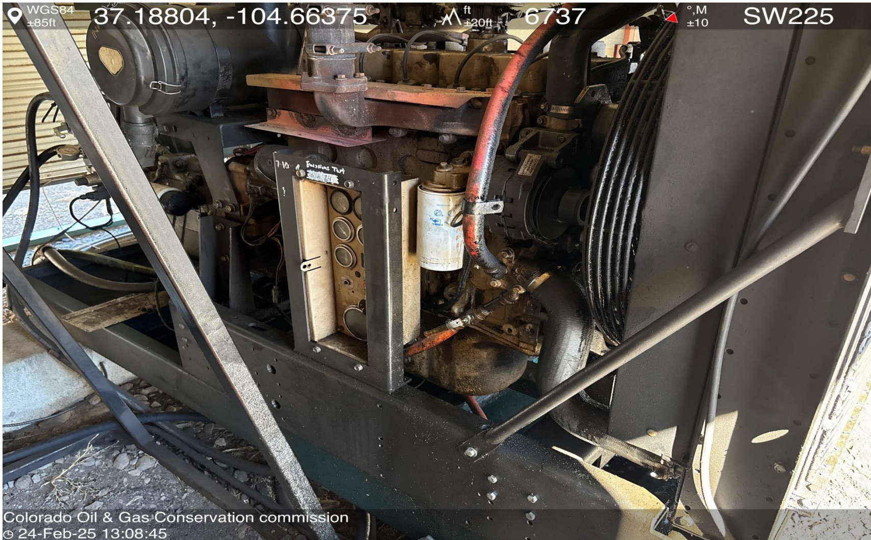
PHOTO 6: MOST OF THE ENTIRE MOTOR AND SKID IS COVERED WITH OIL.
