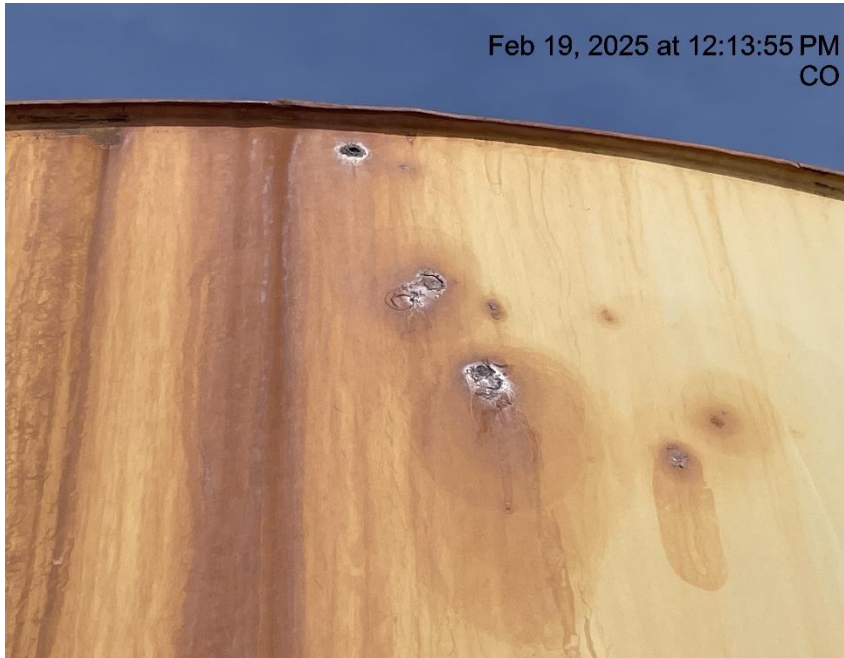
Photo # 6942 Multiple holes in tank/tank lacks integrity
