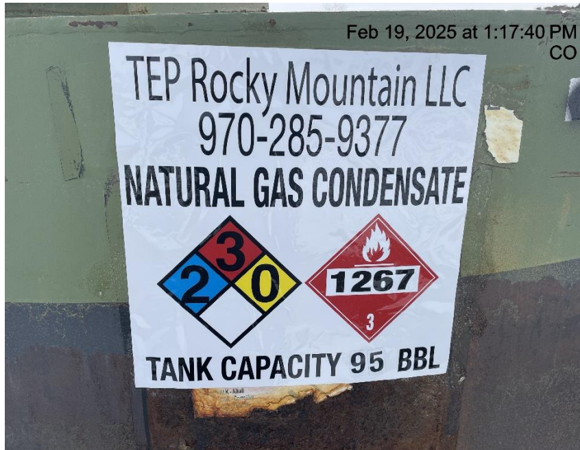
Photo # 7201 Tank capacity incorrect
