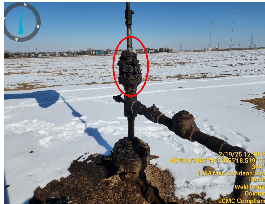
Photo 4: Possible leak, mechanical issue
