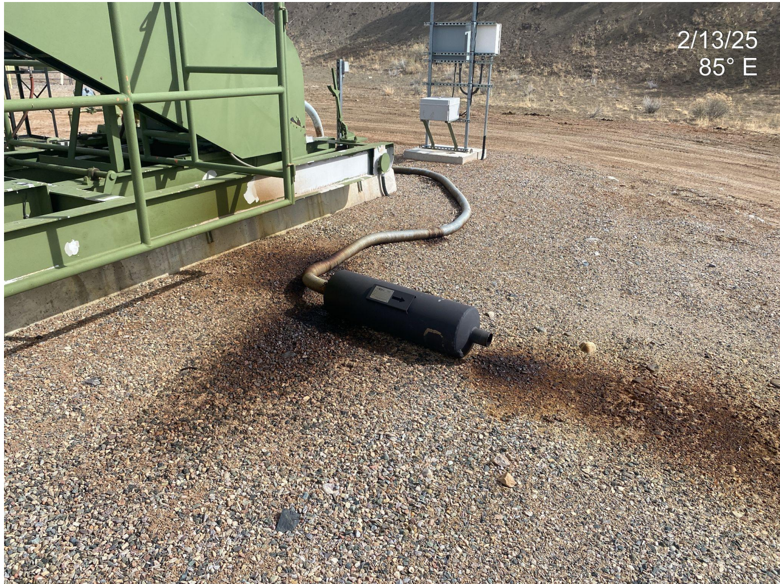
Photo 2. Stained soils at pump jack muffler.
