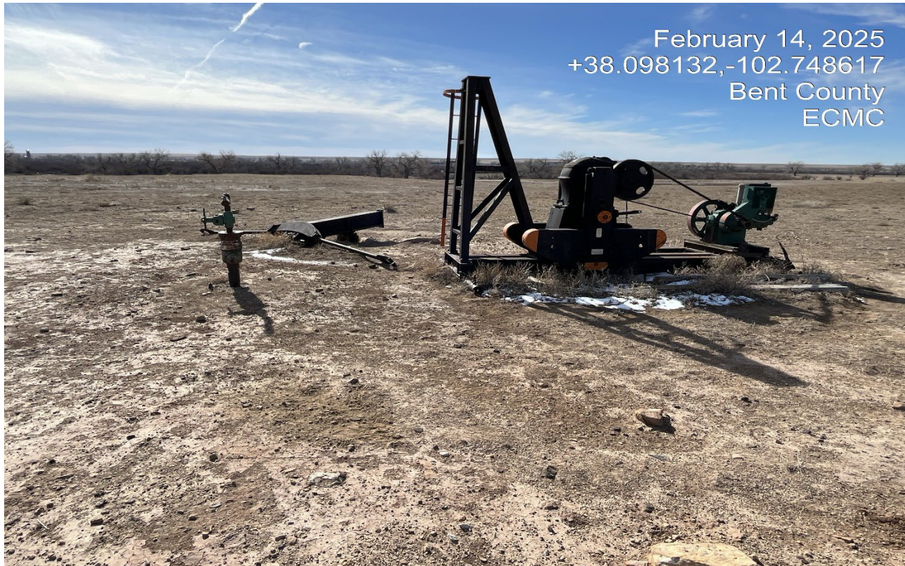
Photo 7. Facing north toward the TA'd well. The pumpjack and parts are unused equipment that need to be removed.
