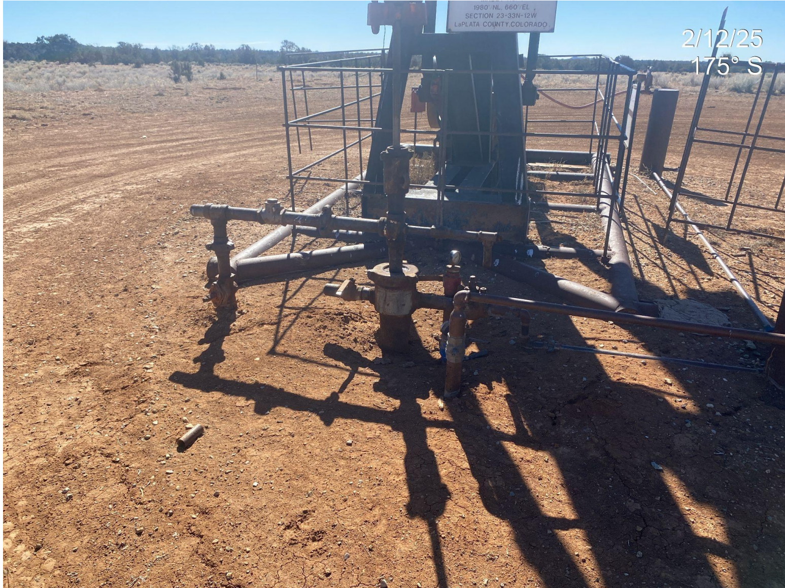
Photo 2. View of wellhead/pump jack, no stained soil was observed.
