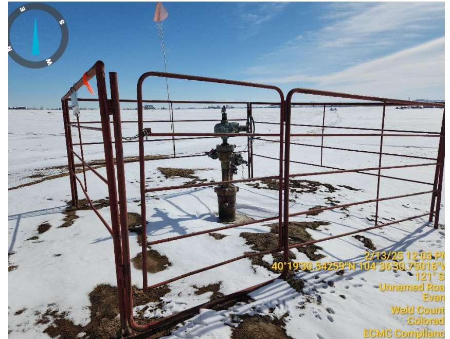
Photo 2: PA wellhead
