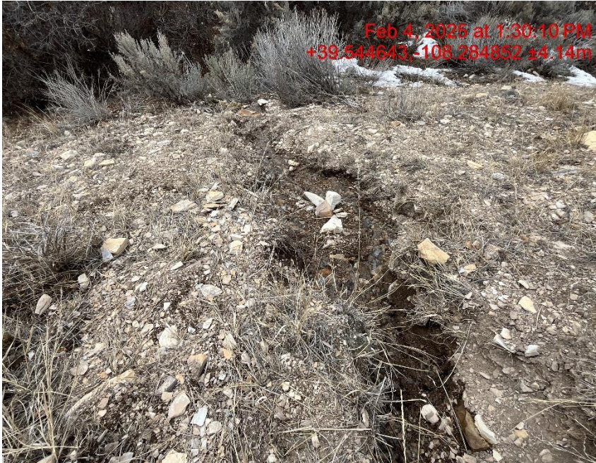
Photo # 4117 Failure to minimize erosion & transport of sediment off location/insufficient BMP's
