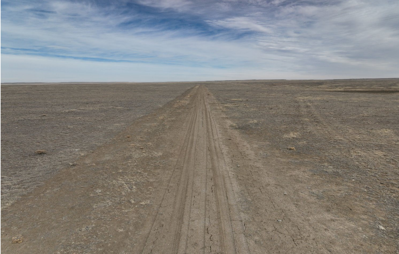
Photo 2. Drone aerial photo facing north along the access road. The former access road has not established perennial vegetation and needs to be reseeded.
