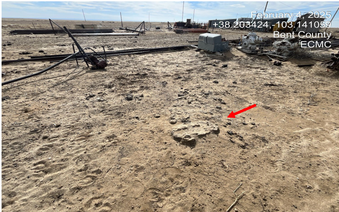
Photo 17. Facing southwest at the location. There are hardened hydrocarbon impacts shown at red arrow.
