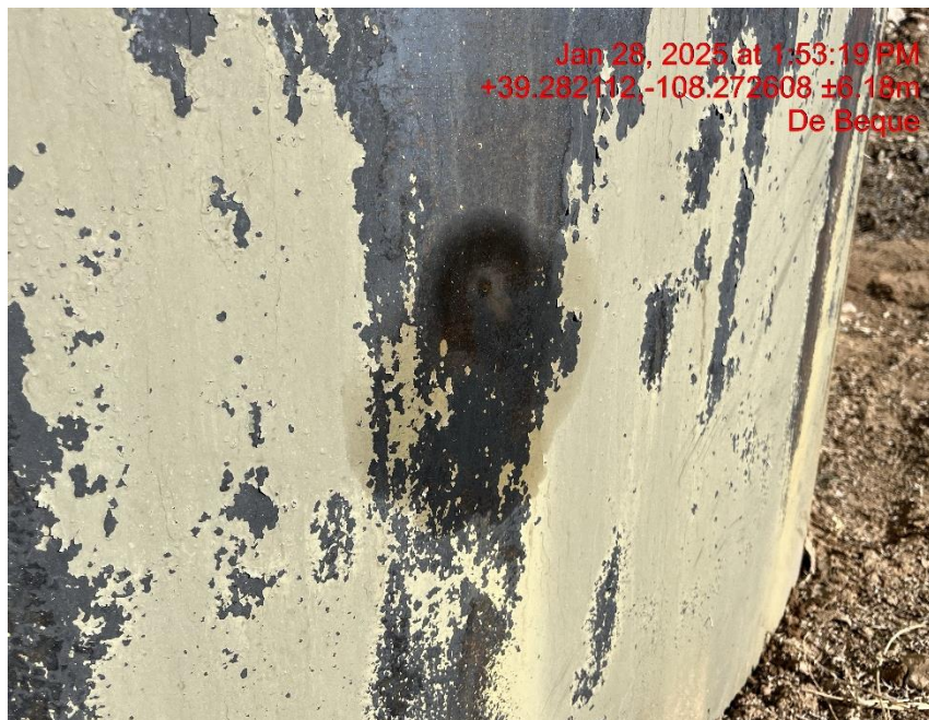
Photo # 3706 Suspected leaks on production tank/tank appears to lack integrity
