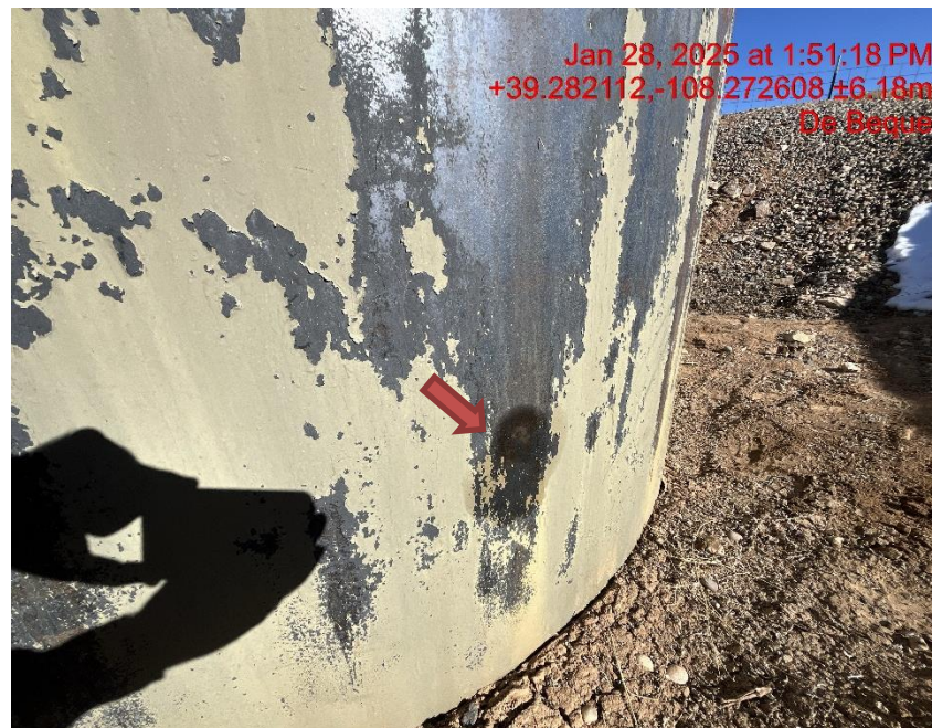
Photo # 3704 Suspected leaks on production tank/tank appears to lack integrity
