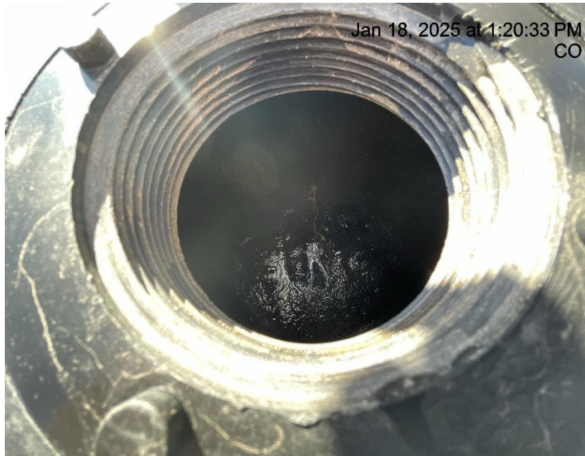
Photo # 360 From inspection 708905502 conducted on 01/18/2025 Failure to maintain chemical BMP – Chemical tank containment approximately 2/3 full of fluid/BMP insufficient to contain possible spill
