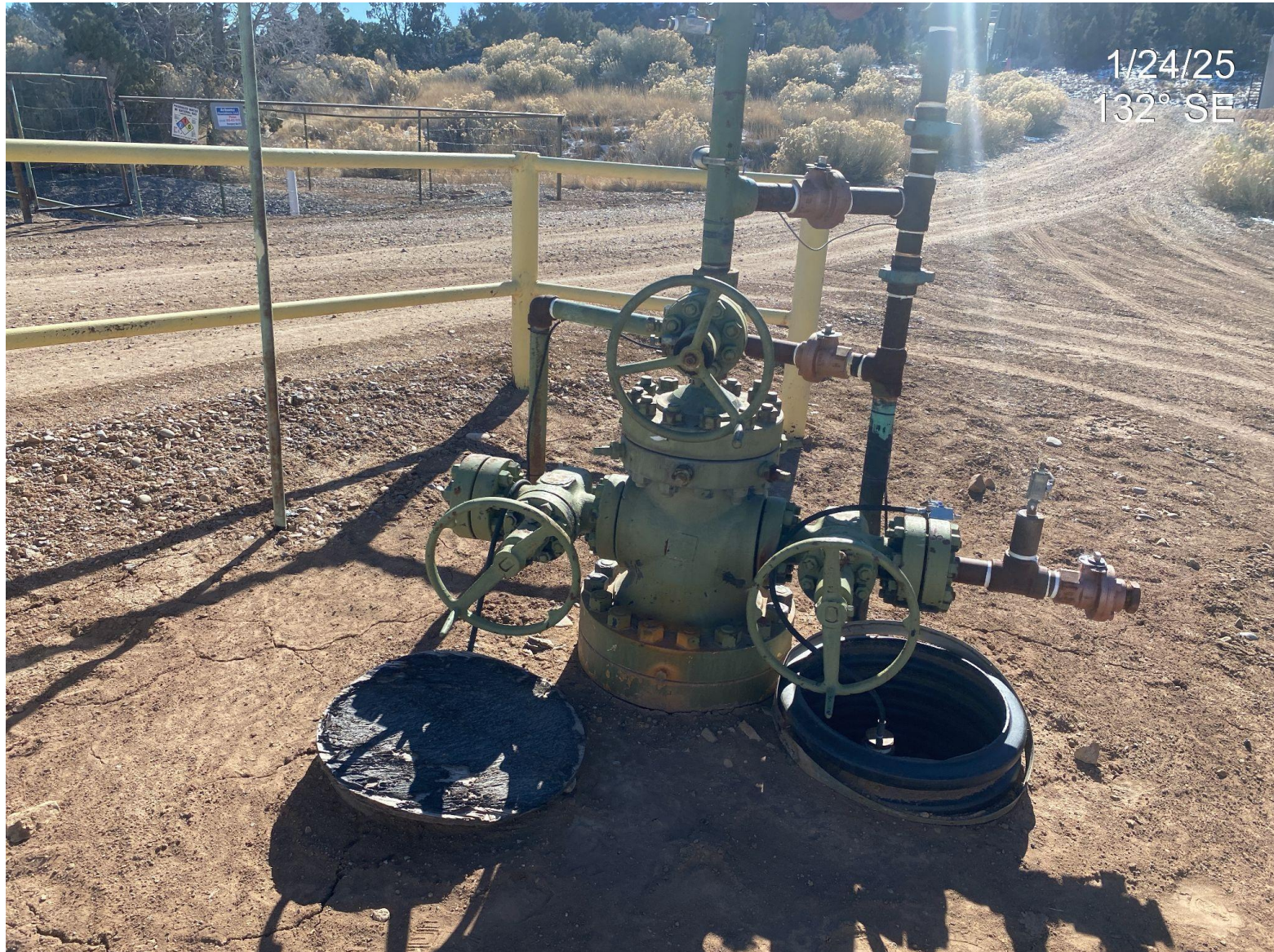
Photo 3. Cellar at well head (#1) is missing wildlife covering/netting.
