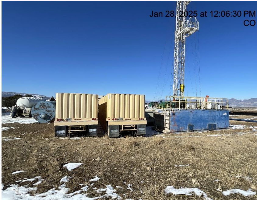
Photo # 1725 Tanks lack secondary containment/failure to comply with COA
