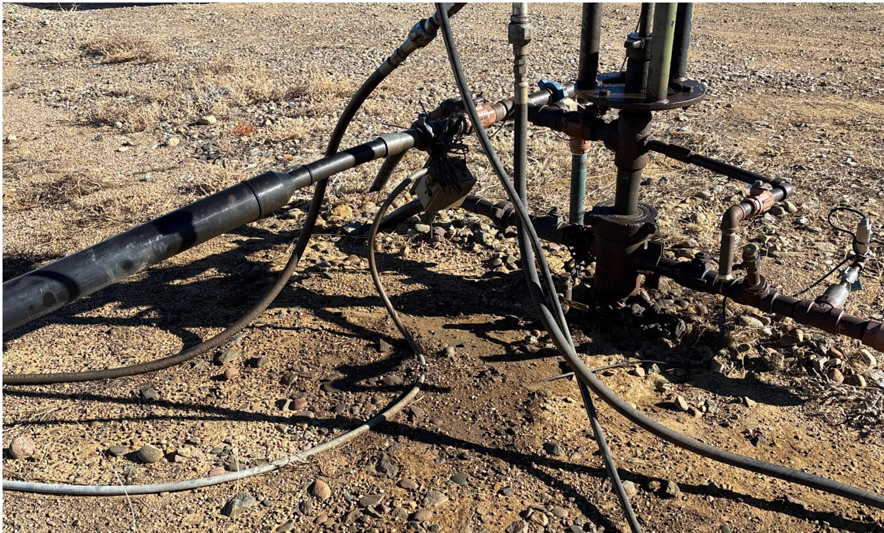
PHOTO 4: AREA OF IMPACTED SOIL AROUND WELLHEAD APPEARS TO BE FROM LEAKING DRIVEHEAD. Conduct maintenance on equipment, cleanup stained material and review self inspection processes. COMPLY WITH RULE 1002,(2).D. CA DATE 1-10-2025.
