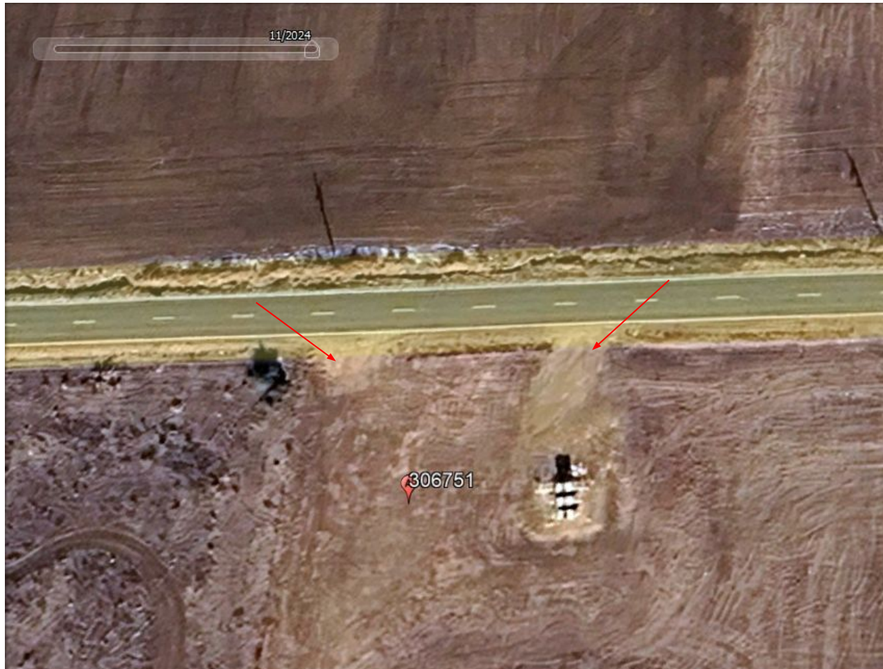
Photo 5. Google Earth aerial imagery (circa 11/2024) illustrating that the two tank battery entrances remain and will require additional reclamation activities. Meter sheds pictured have been removed at the time of this inspection.
