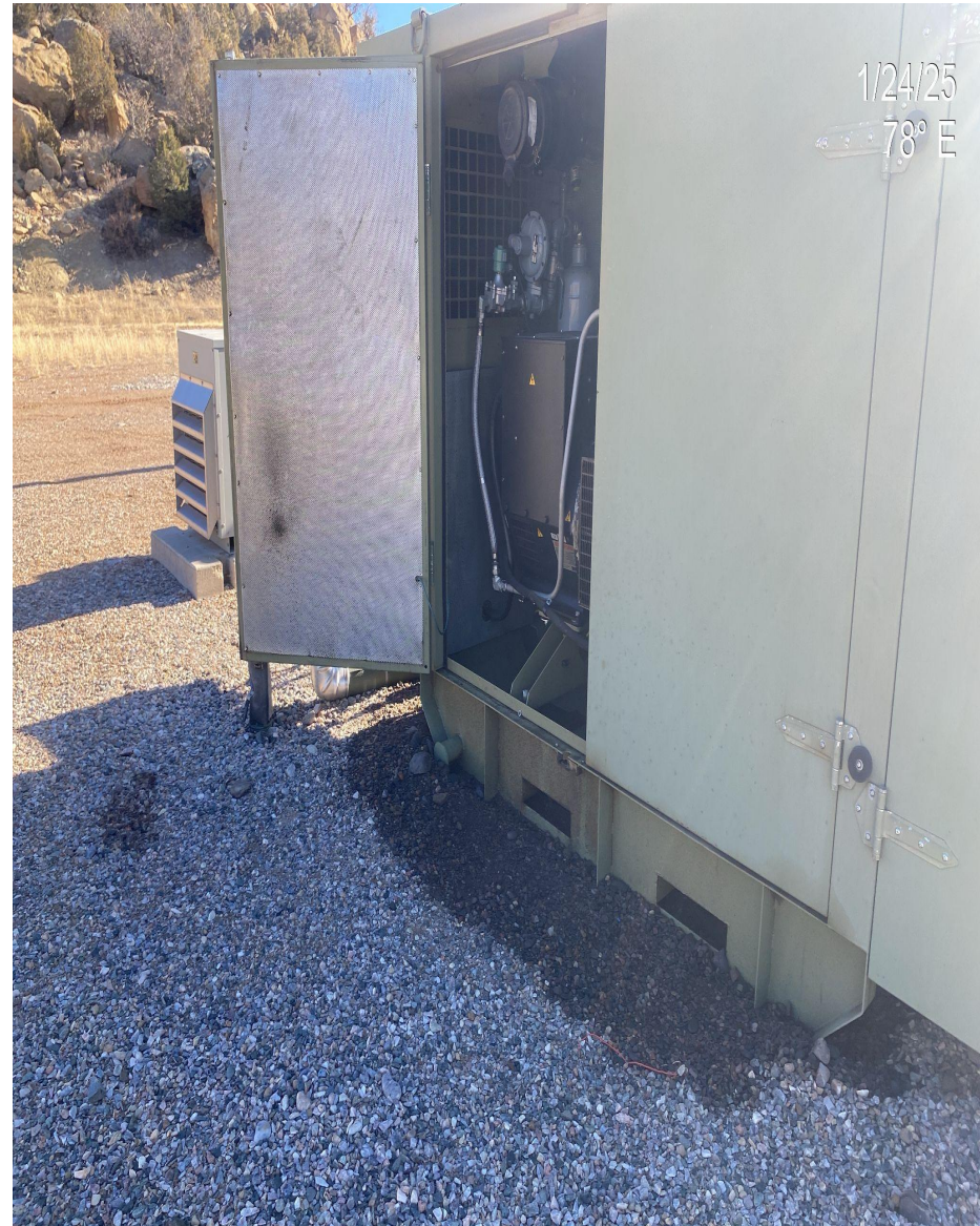
Photo 2. Stained soils at oillift equipment.
