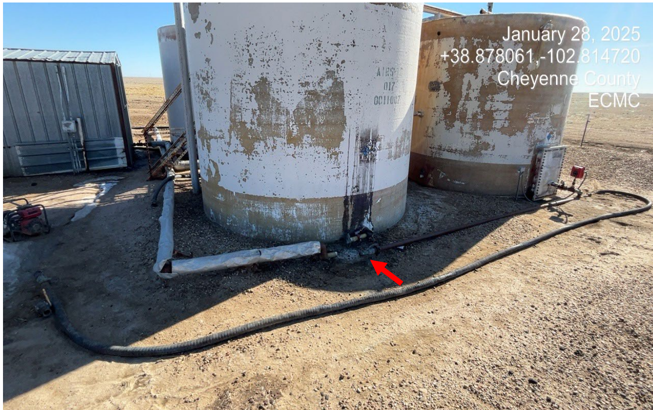
Photo 10. It appears the fiberglass tank at the west side also leaked fluids.
