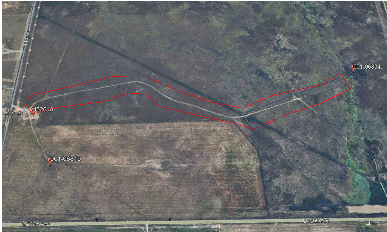
Photo 9. Aerial Photo from google 09/2023. All wells being serviced by main access road are plugged and abandoned. Vegetation has not established on access road. Main access road appears to require further reclamation (red circle).
