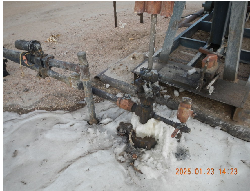
2. View of wellhead. Well leaking at packing at time of inspection.
