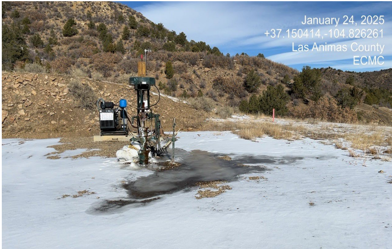
Photo 2. There was a water leak at the wellhead.
