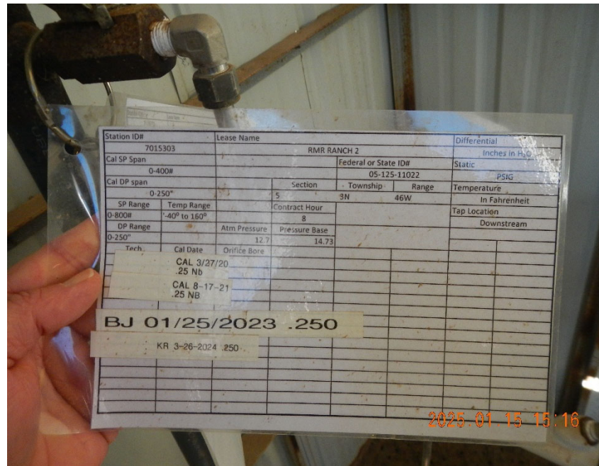
8. Calibration log with incorrect well API number.
