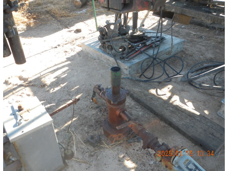
2. View of wellhead. Rods removed.
