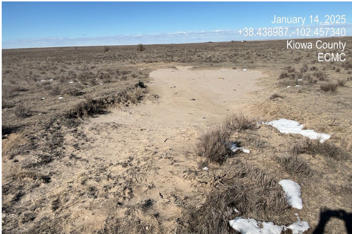
Photo 8. Just north of the wellsite (~500') is another impacted area with no vegetation establishment and erosion.
