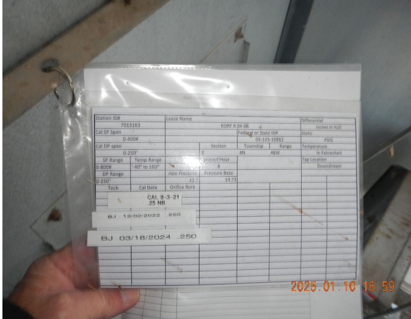
5. Calibration log with incorrect API number.
