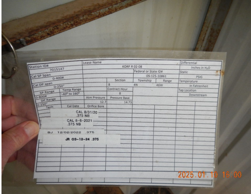
7. Calibration log with incorrect API number.
