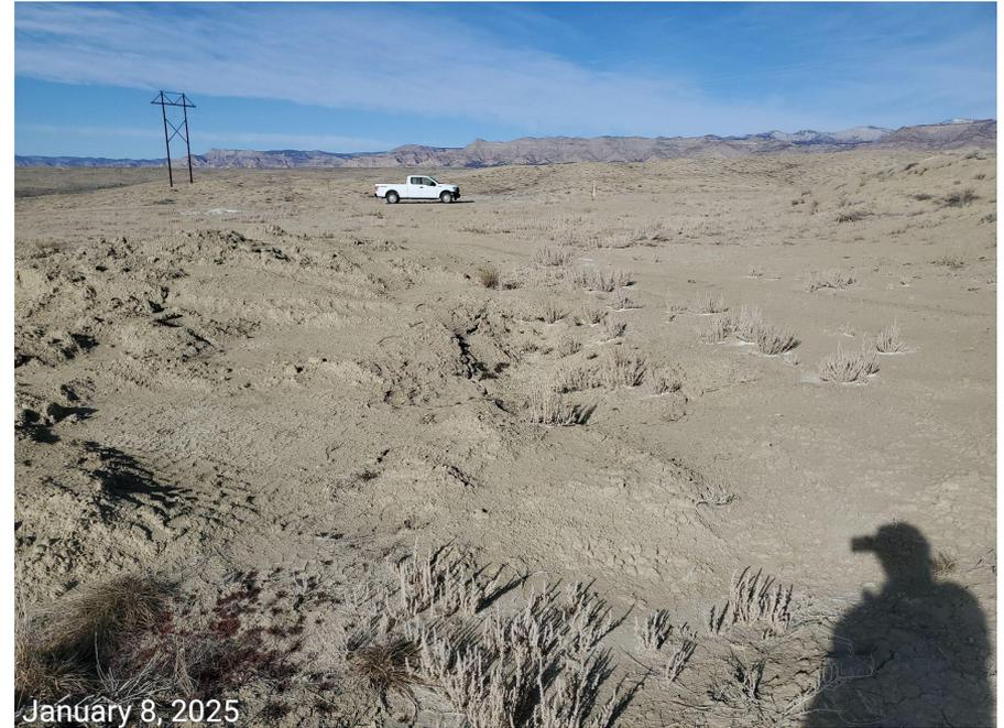
**Photo 3:** Photos taken from the south end of the Location. Photos provide an overview of the Location from northwest to north. Photos show final reclamation has not been performed in accordance with 1004 requirements- Location has not been decompacted, recontoured/regraded and reclaimed; Undesirable and Noxious Plant Species (Halogeton) observed established throughout the Location disturbance.
