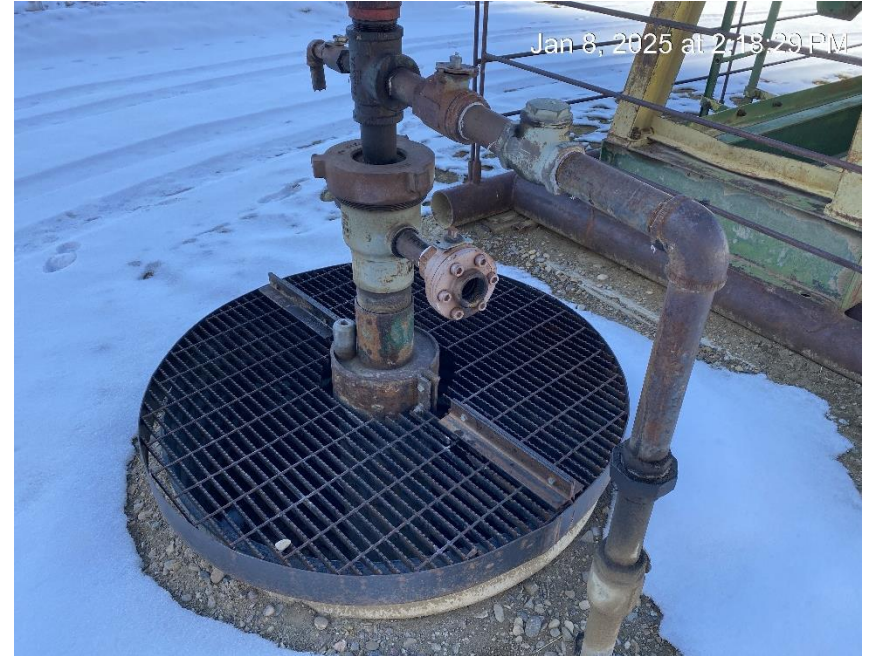
Casing venting to atmosphere. LEL meter confirmation.
