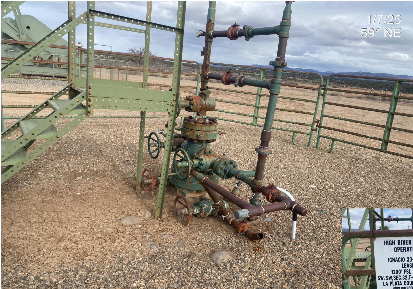
Photo 1. View of wellhead assembly. Well sign missing local emergency services number.
