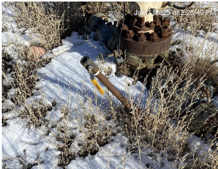
Discovered surface valve in open position
