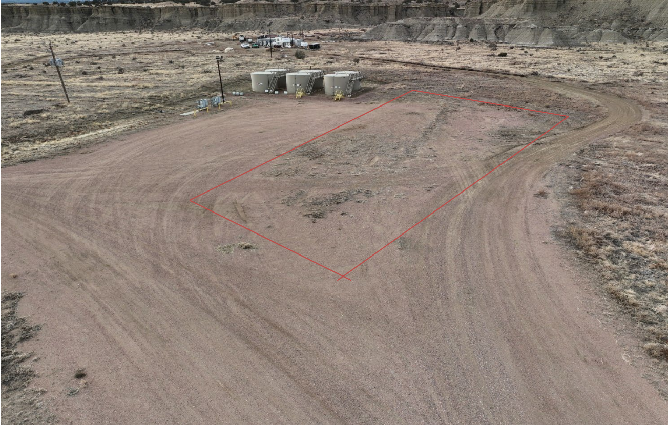
Photo 1. Drone aerial photo facing southwest overlooking the abandoned wellsite and active tank battery. The highlighted area of the abandoned wellsite has not been reclaimed.
