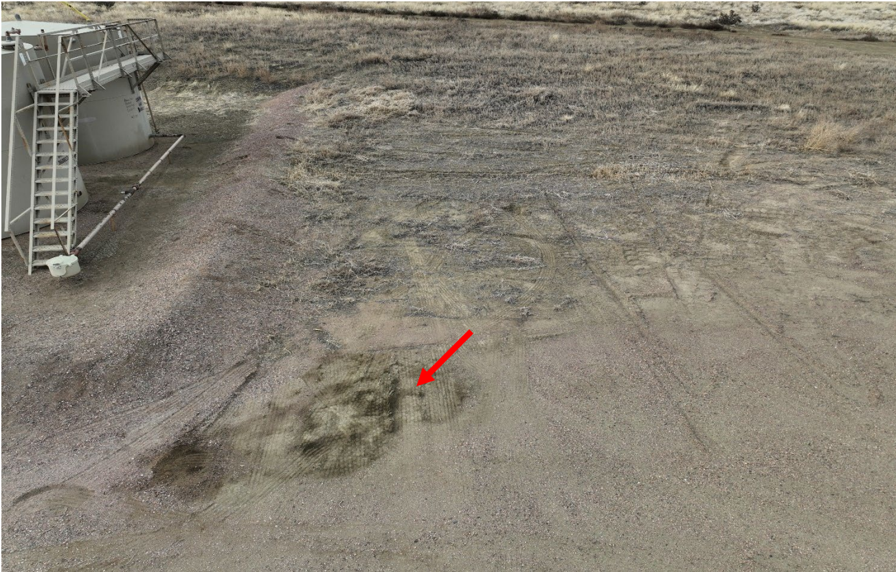
Photo 5. It appears a recent truck load out has spilled oil onto the ground at red arrow. The oil stained soils must be cleaned up.
