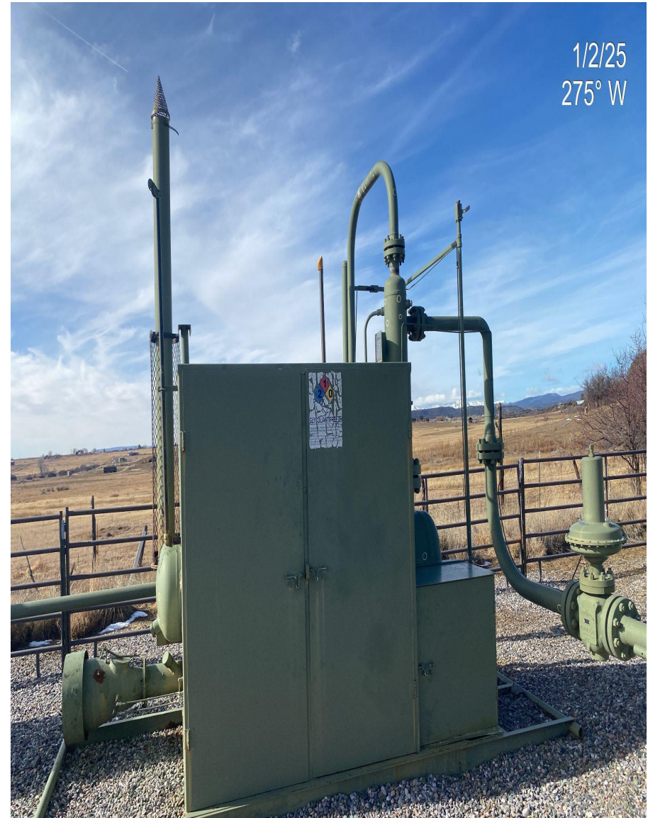
Photo 3. Signs/Placards at separator have deteriorated and are no longer legible.
