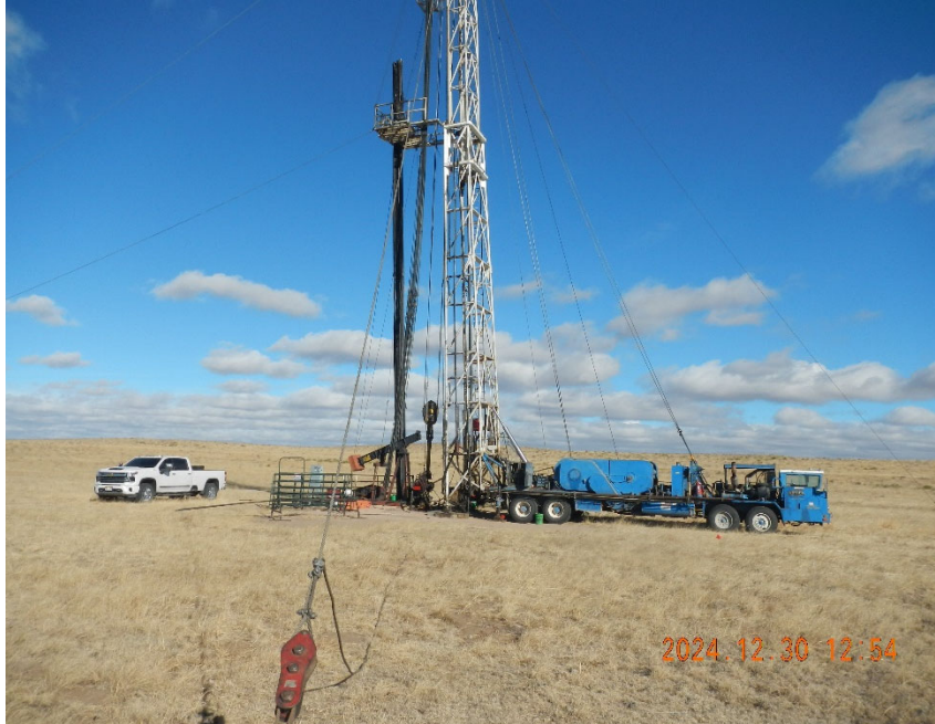
3. Rig set up over well.
