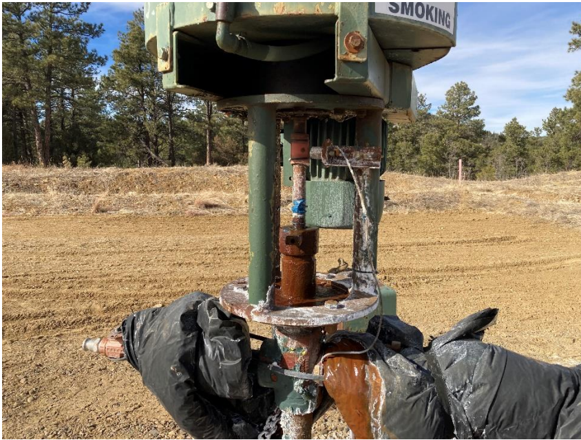
Photo 5 – Leaking packing at 41-30 wellhead
