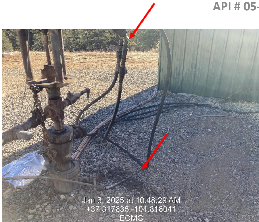
Photo 7 – Hydraulic fitting on wellhead leaking, stained soils
