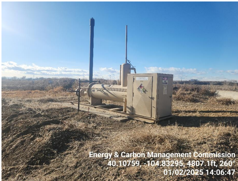
Photo 7 Horizontal Heated Separator.
