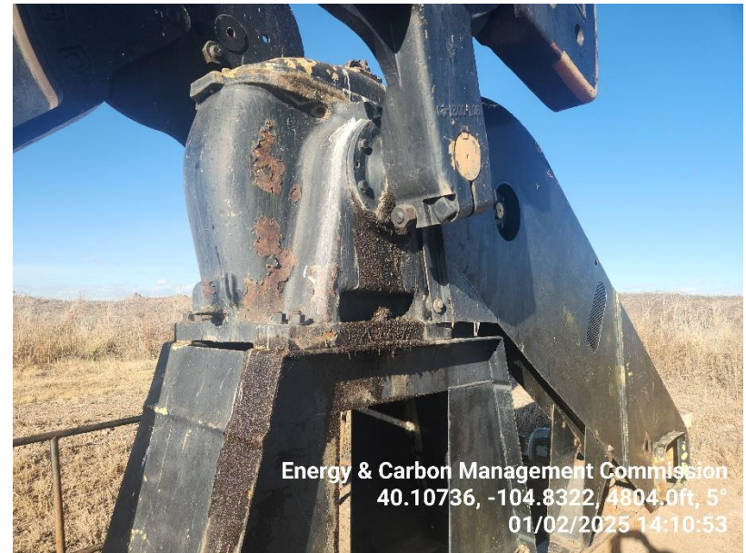
Photo 14 Leaking gear box.
