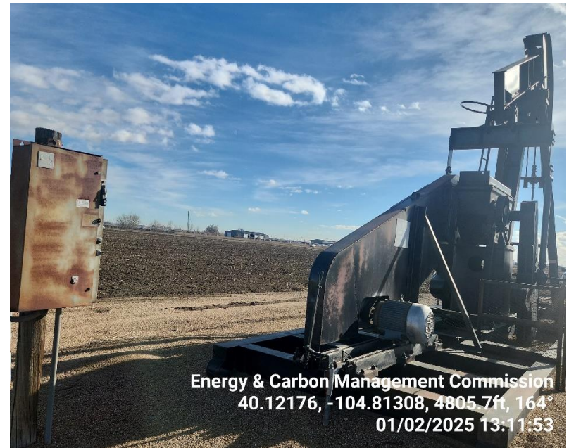
Photo 4 Electric panel, electric motor & pump jack.
