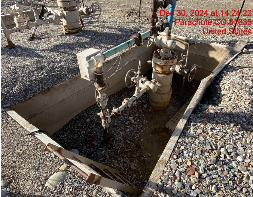
Open Wellhead Cellar – Photo #05664
