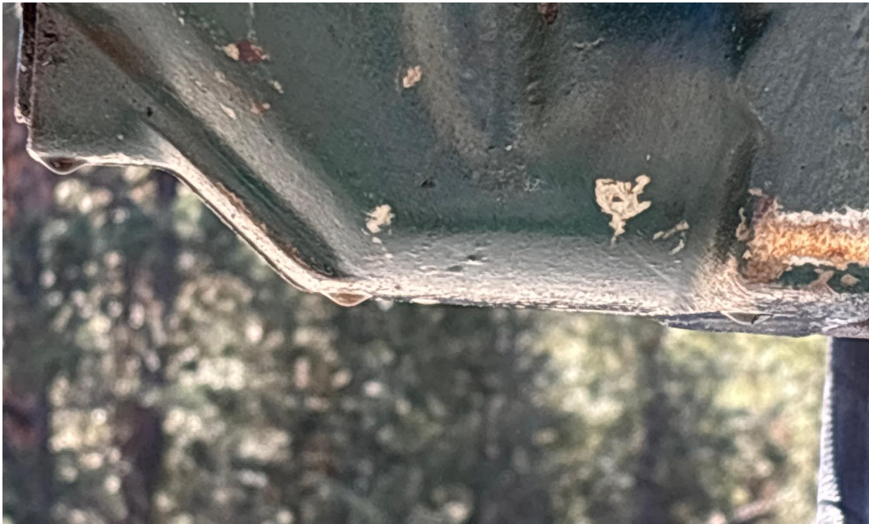
PHOTO 6: DRIVEHEAD MOTOR LEAKING HYDRAULIC OIL. REPAIR EQUIPMENT PER RULE 606. CA DATE 1/9/25.
