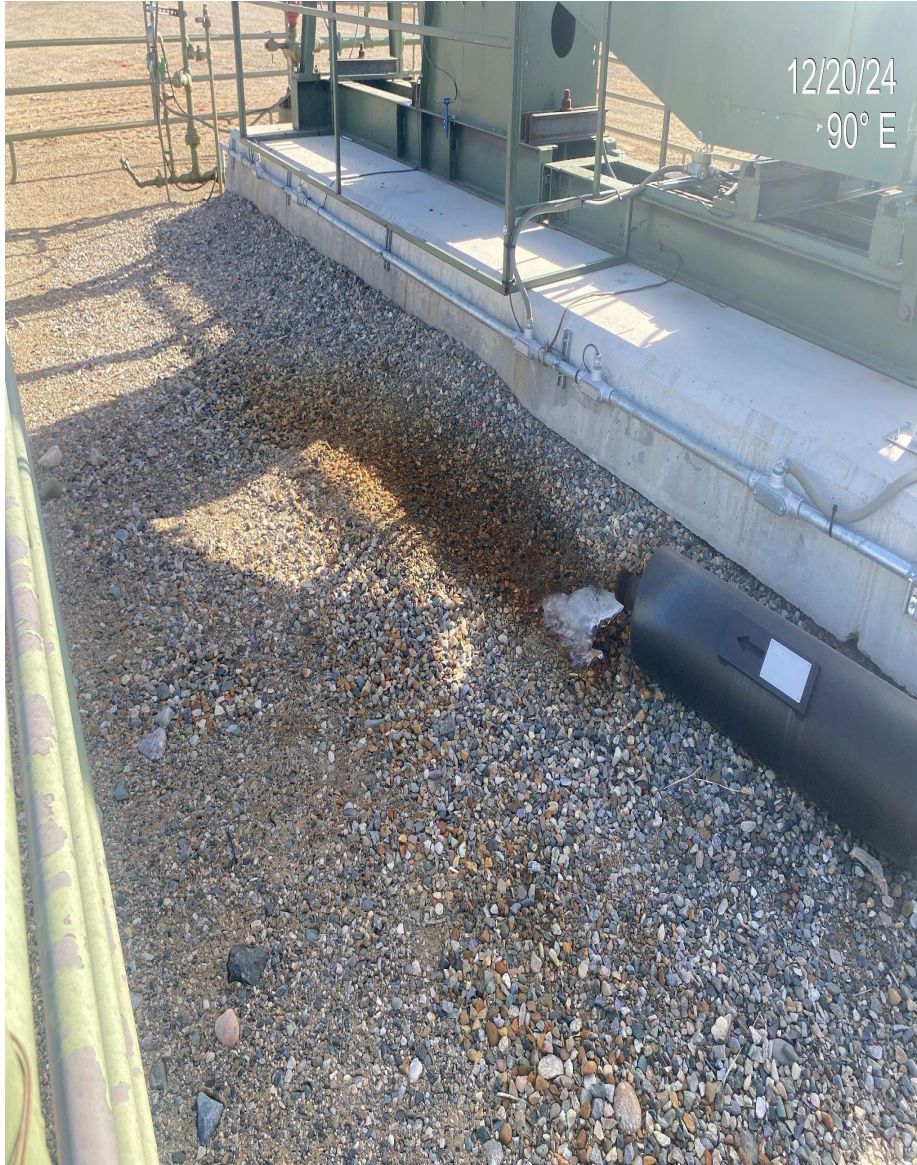
Photo 3. Impacted material at well head and pump jack muffler.
